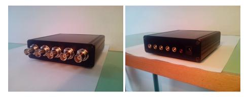
Figure 3.26: The preamplifier module: (Left) BNC Inputs, (Right) Lemo outputs
