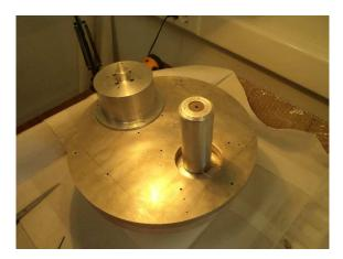
Figure C.14: Preparation for disassembly of the HDA. Although the analyser is made of large parts, there is a great number of tiny insulating sapphire balls, so extra caution is needed during this procedure.
