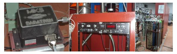
Figure 3.9: Gas delivery system. From left to right: MKS 390H pressure transducer, MKS 250E pressure controller and MKS 270D signal conditioner and last, the gas manifold.
