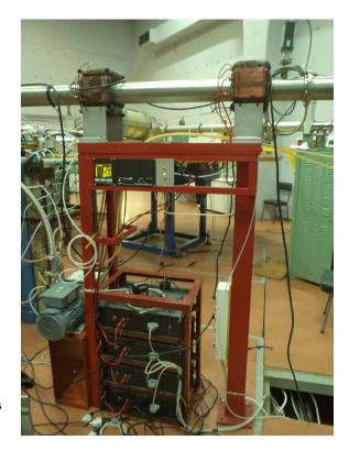
Figure C.3: Electromagnetic steerer coils and dedicated current supplies.
