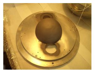
Figure C.15: Disassembly of the HDA. The carbon coated hemisphere is the inner sphere  $V_1$  electrode. Beneath it, is located the plate electrode on potential  $V_p$ . The lower hole corresponds to the entrance of the analyser, and the upper hole to the exit. The HDA electrodes are stacked on the support plate and electrically isolated to about 5kV using sapphire balls of various radii.
