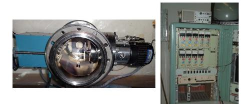
Figure C.5: (Left) Photo of the inside of the Beam Profile Monitor (BPM) depicting motor and shaft of the rotating wire. The metal shield lining the inside of the beam-line is connected to the BPM signal collector. (Right) Photo of BPM controller box (down just above Nuclear Instrumentation Module (NIM) crate) and on top the oscilloscope viewer at the Tandem control console.
