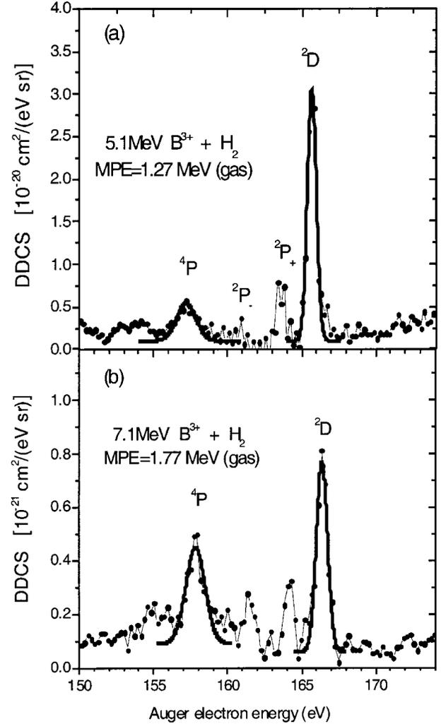
FIG. 2.  $0^\circ$  Auger spectra measured for  $\text{B}^{3+} + \text{H}_2$  collisions at the projectile energies of 5.1 and 7.1 MeV. The  $\text{B}^{3+}$  ( $1s^2\ {}^1S, 1s2s\ {}^3S$ ) beam was obtained in collision of primary B with nitrogen gas at the metastable production energies (MPE) of 1.27 and 1.77 MeV, respectively.
