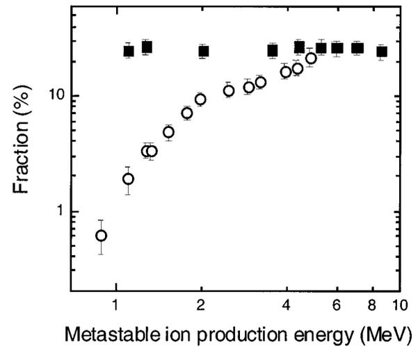
FIG. 4. The metastable fraction  $F = B^{3+}(1s2s^3S) / B^{3+}(1s^2 1S, 1s2s^3S)$  versus the stripping energy. Circles, the metastable fraction of the ionic beam produced in  $N_2$  gas; squares, the metastable fraction of the ionic beam produced in carbon foils. The error bars correspond to the statistical uncertainty and are plotted at the 90% confidence level.
