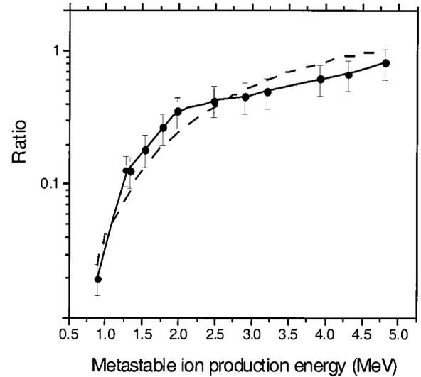
FIG. 5. The comparison of predicted and observed ratios of the metastable fraction produced in gas to the metastable fraction produced in a foil. Circles, experimentally observed ratio of metastable fractions,  $F_{\text{gas}}/F_{\text{foil}}$ . Dashed line, the ratio predicted by the proposed model,  $M_1/N_1$ .
