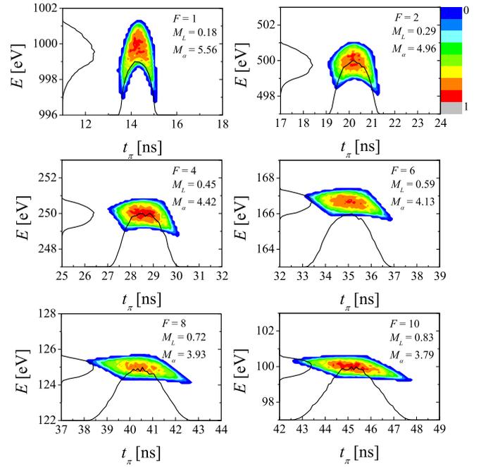
**Fig. 2.** Calculated time and energy distributions at the exit of the HDA for six different values of  $F = 1 - 10$ , for a monoenergetic beam of  $E_{s0} = 1000$  eV. Simulations were performed for a source extent of  $d_s = 2.5$  mm. Normalized line profiles resulting from vertical and horizontal projections of the distributions are also shown. The detector plane is assumed to coincide with the HDA exit plane.
