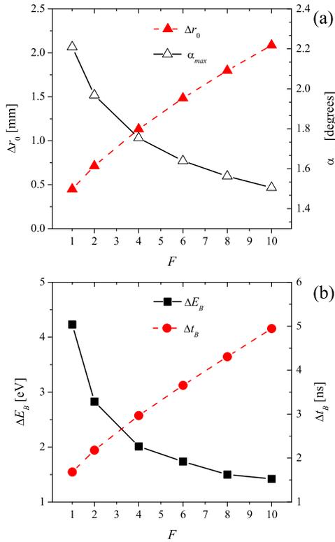
**Fig. 3.** (a) The values of the virtual entry aperture size  $\Delta r_0$  and the angular spread  $\alpha_{max}$  computed by the lens magnification  $M_L$  and angular magnification  $M_x$  according to the Helmholtz–Lagrange stipulations plotted as a function of  $F$ . (b) Comparison of the base energy  $\Delta E_B$  and time  $\Delta t_B$  spread as a function of  $F$ .
