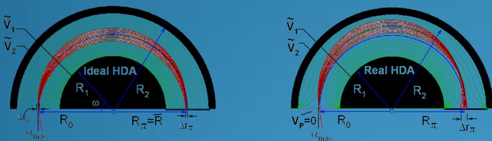
Fig. 1. Electron trajectories in an ideal and a fringing field HDA
