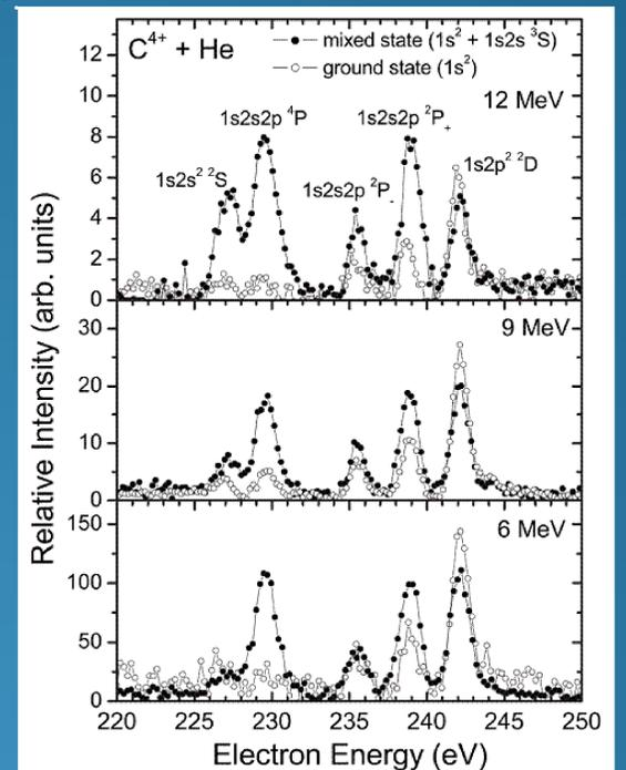
Fig.3 K-Auger spectra from mixed and pure ground state  $C^{4+}$  beams at three collision energies<sup>4</sup>
