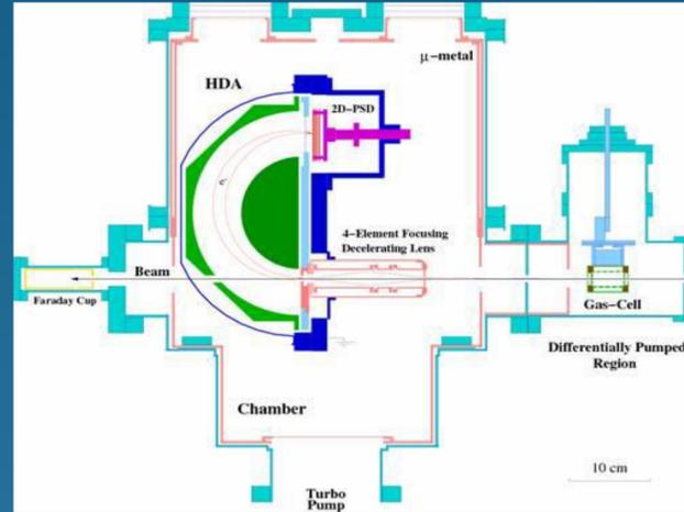
Fig.2 Proposed Zero degree Auger Projectile Spectroscopy experimental setup.
