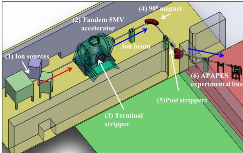
Figure 1: The TANDEM accelerator laboratory of the NCSR “Demokritos” and the APAPES experimental station. The position of the three new strippers is indicated.
