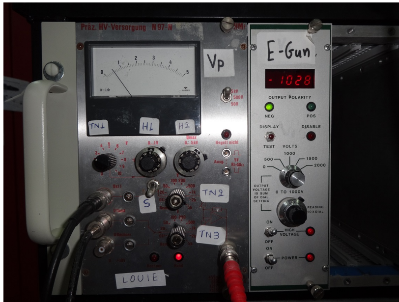
Figure 1: HMI and Tennelec HVPSs assigned for the voltage on the V_2 electrode and the hot wire electron gun respectively.
